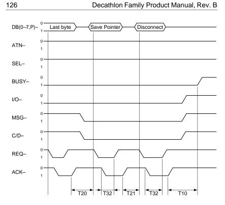
Figure 22. Last data byte, save pointer message and disconnect message
