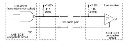
Figure 2. Singled-ended transmitter and receiver
