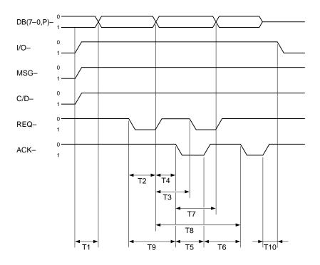
Figure 25. Synchronous write timing
