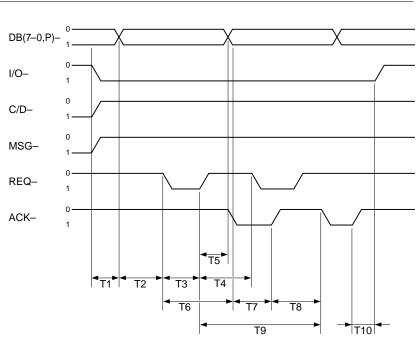
Figure 24. Synchronous timing
