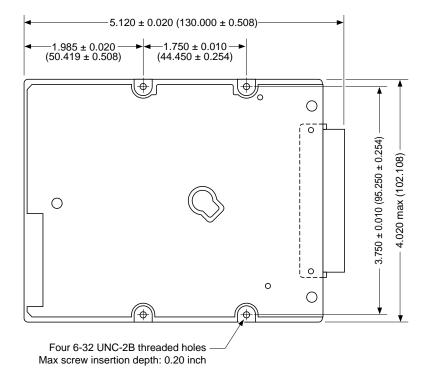
Figure 8. ST5660NC mounting dimensions
