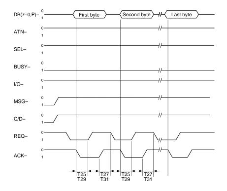
Figure 21. Data out block transfer
