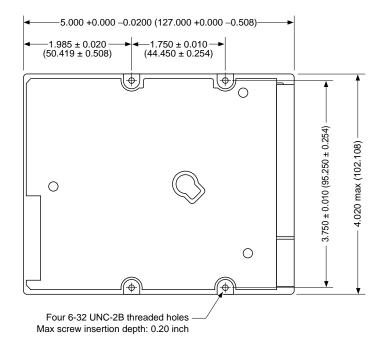
Figure 7. ST5660N mounting dimensions
