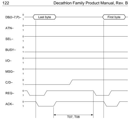
Figure 18. Last command byte to data out
